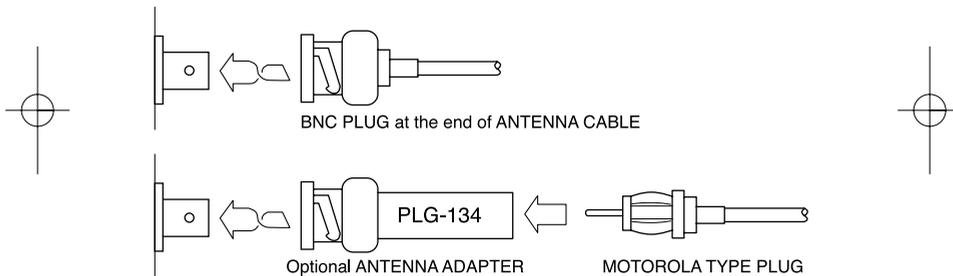
Connect your Antenna plug here. If you have a Motorola-type plug, use the optional adapter (PLG 134).
